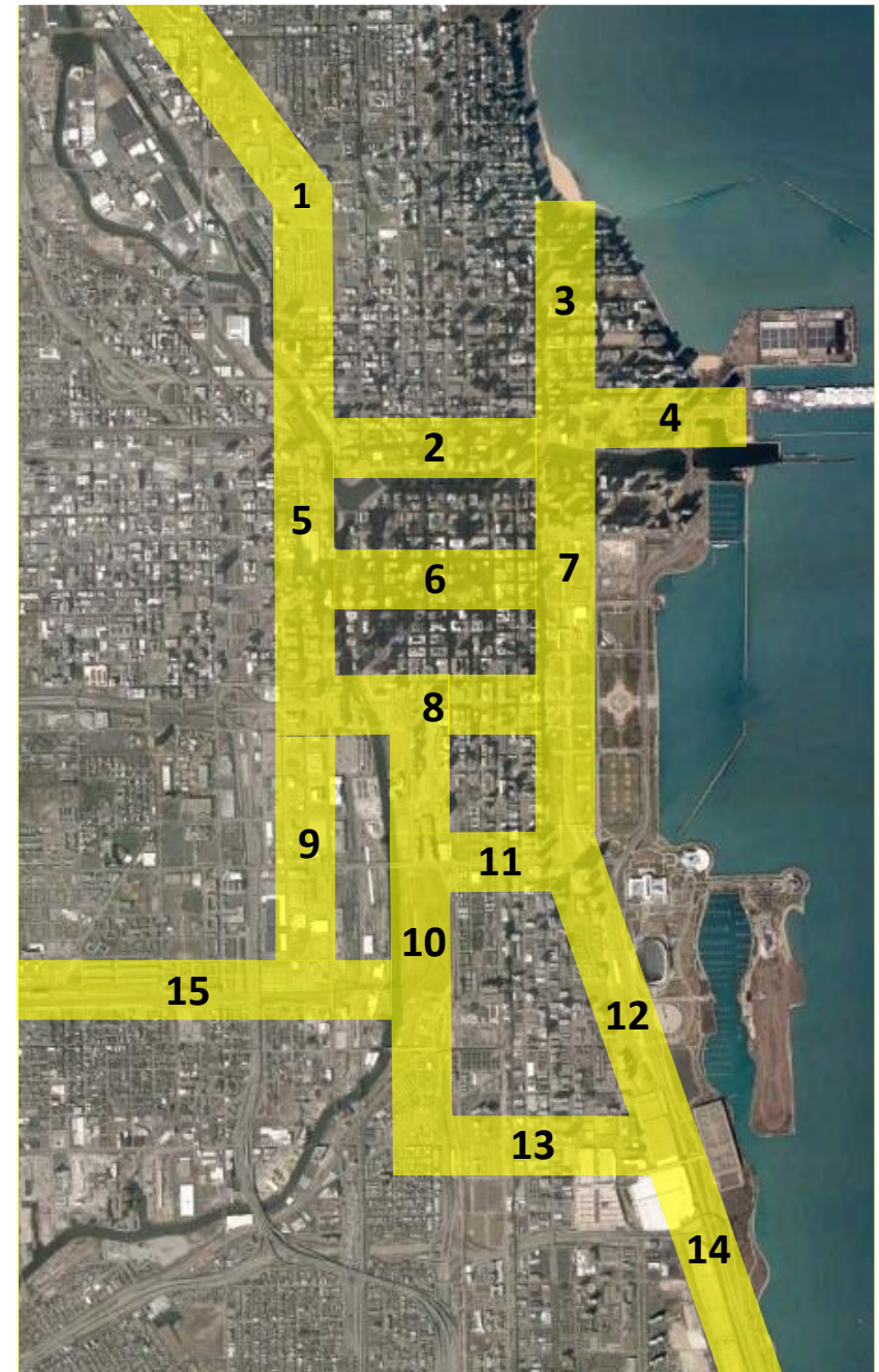
Figure E-15. Potential rail corridors
